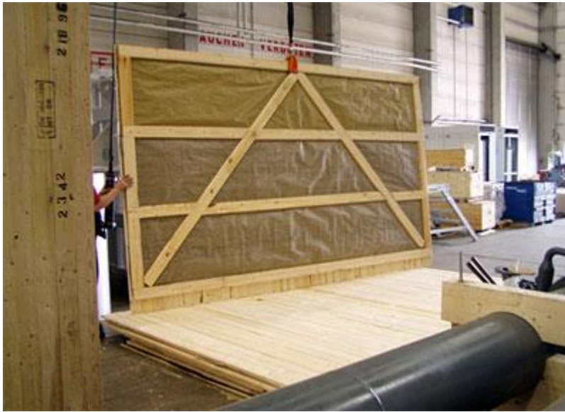
Figure 6: Side wall lined with a barrier layer
